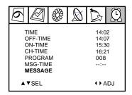
Press **VOL+/-** to access the MESSAGE interface. Press **MENU** button to enter words and symbols. You can enter four lines at most and each line is composed by 15 letters or symbols.
